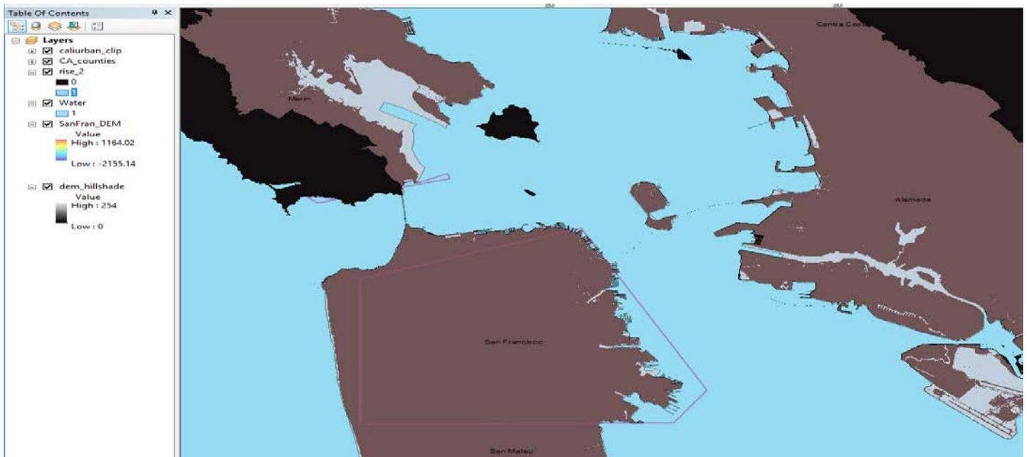
**Figure 15:** Raster calculation added to ArcMAP representing a sea level rise of 2 meters.
