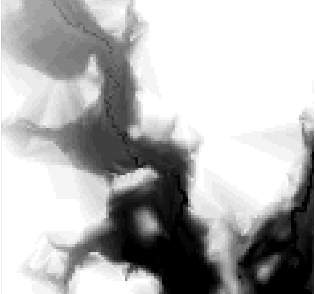
Figure 13. Default cell size 250 feet raster showing very coarse resolution
