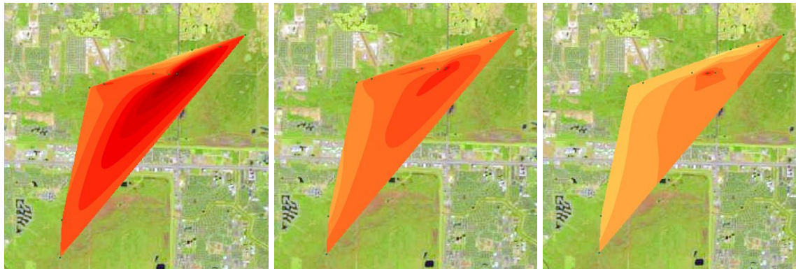
Figures J, K1, K2, K3 - Window with manual classification method, creating classes every 0.1 with “break values”. Bottom set of figures (K1-3) is the same data under 16 class scheme, with 2 cm in the far left and 30 cm on the far right, with dark red indicating high RQ values (1.5-1.6) and pale yellow indicating low RQ values (0.0-0.1), with red indicating the estimated global average (0.9-1).
