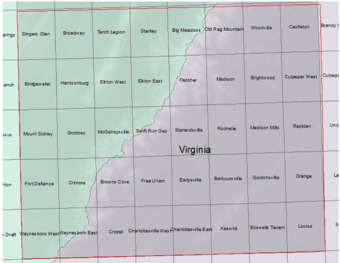
Figure 5: The Area of Interest created from the Create Features tool. The light green polygon is the 207 subregion of the HU-4 Basin for the NHD Hydrography dataset. The light purple polygon is the 208 subregion of the HU-4 Basin for the NHD Hydrography dataset. The “ major_rivers ” shapefiles for these subregions were turned off for this screen capture to reduce clutter and to make the Area of Interest more visible.
