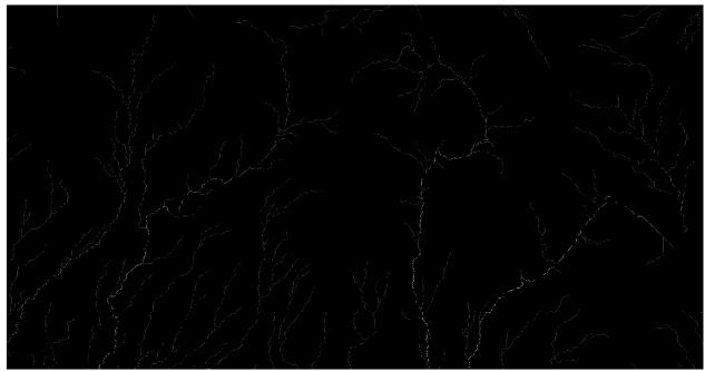
Figure 13. Flow Accumulation. A ranking of how powerful flow is based on how many streams discharge into a single stream. The brighter the line or area, the greater the flow. The symbolization has been enhanced for visual
