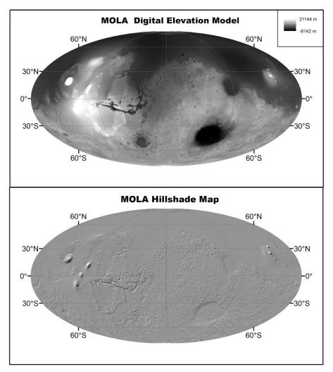
Figure 1. (Top) DEM from MOLA shotpoints. (Bottom) Hillshade map created from MOLA DEM. Both maps have a Mollweide Auxiliary Sphere projection with a GCS Mars 2000 coordinate system.
